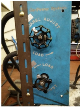
Fig. 11 - Water valves to control the braking force
